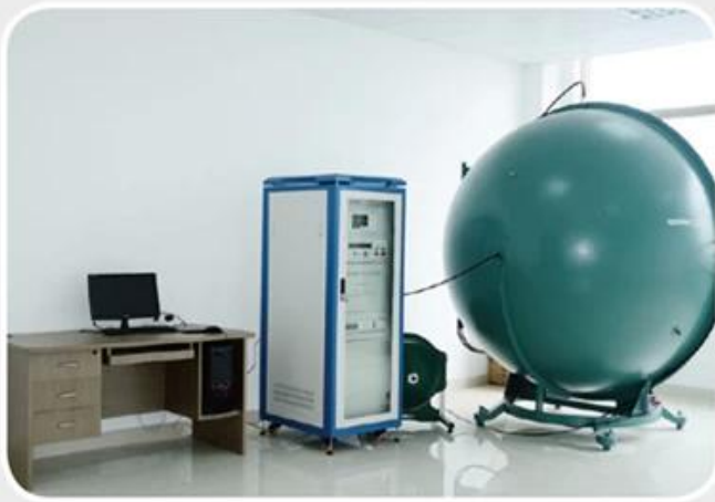
ullbrich sphere for testing luminous flux
