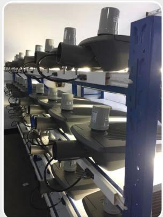
led street lighting aging testing line.
