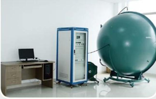
ullbrich sphere for testing luminous flux
