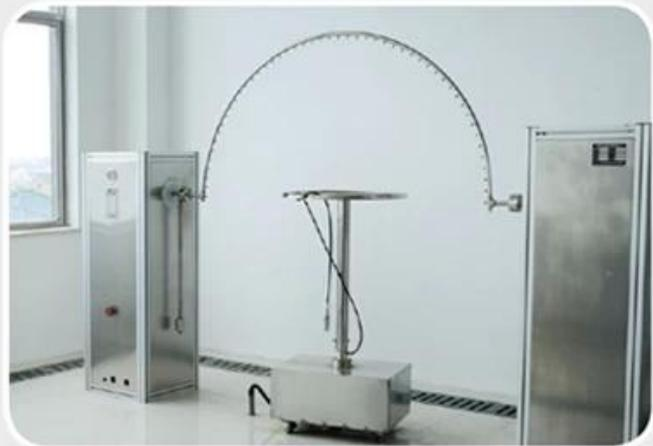
ingress protection (Ip) testing equipment.
