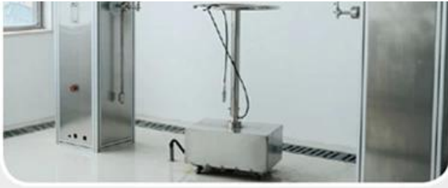
ingress protection (Ip) testing equipment.
