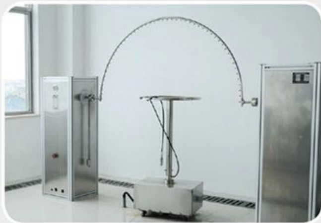
ingress protection (Ip) testing equipment.
