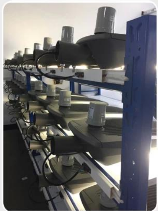
led street lighting aging testing line.
