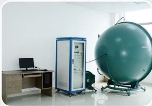
ullbrich sphere for testing luminous flux
