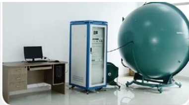
ullbrich sphere for testing luminous flux
