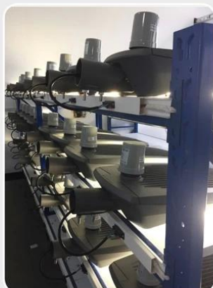
led street lighting aging testing line.
