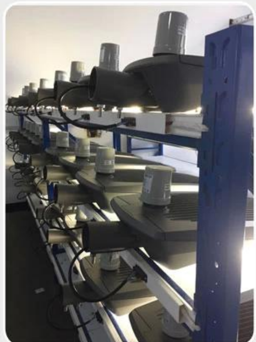
led street lighting aging testing line.
