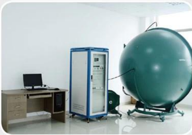
ullbrich sphere for testing luminous flux
