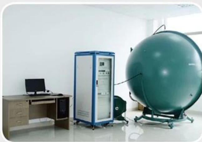
ullbrich sphere for testing luminous flux
