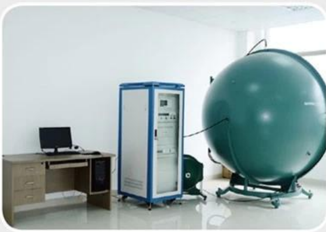
ullbrich sphere for testing luminous flux
