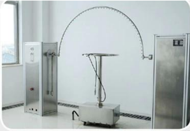
ingress protection (ip) testing equipment.
