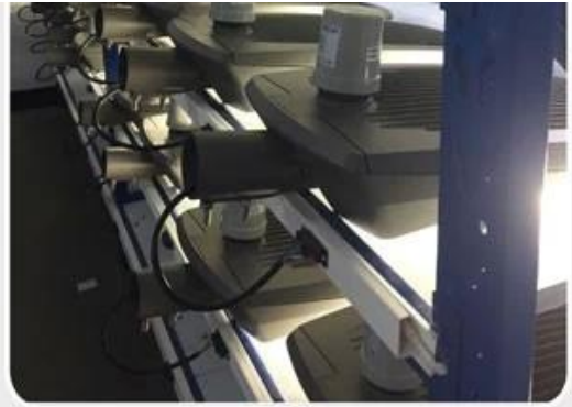
led street lighting aging testing line.
