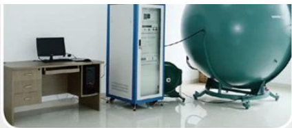
ullbrich sphere for testing luminous flux
