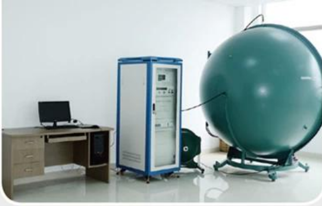
ullbrich sphere for testing luminous flux
