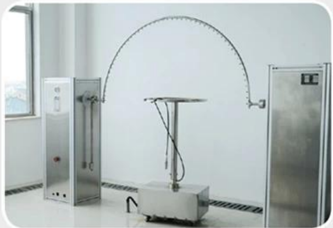
ingress protection (ip) testing equipment.
