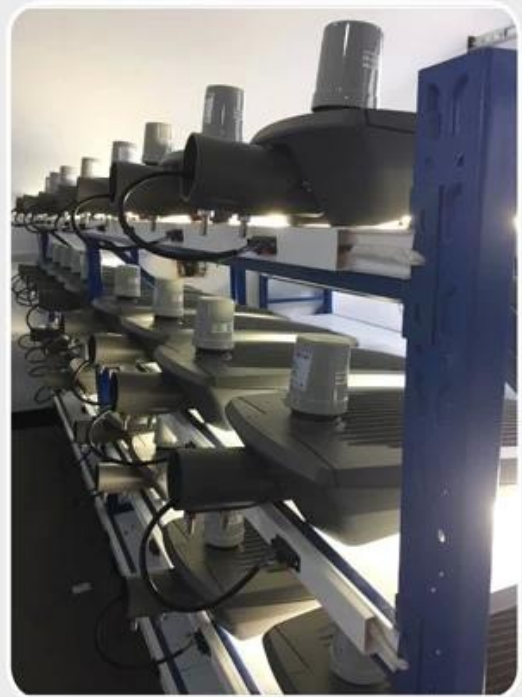
led street lighting aging testing line.
