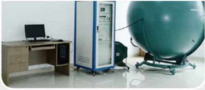
ullbrich sphere for testing luminous flux
