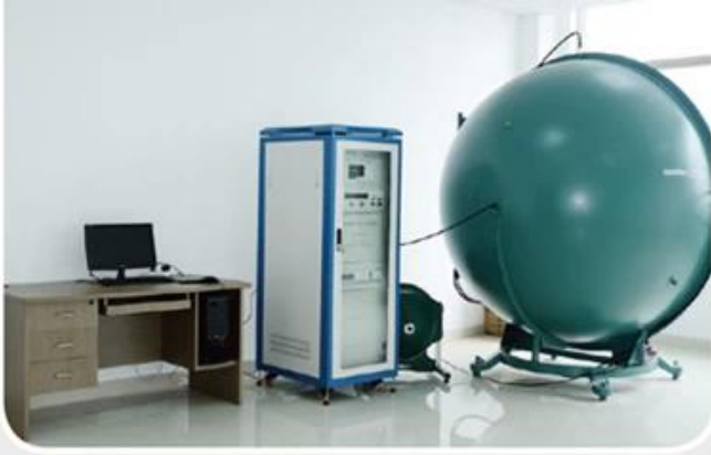
ullbrich sphere for testing luminous flux
