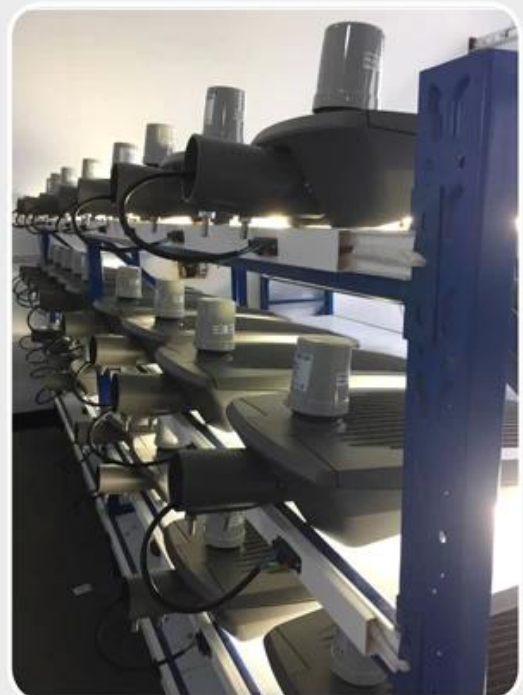
led street lighting aging
