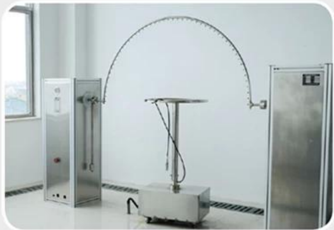
ingress protection (Ip) testing equipment.
