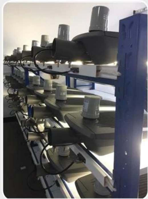
led street lighting aging testing line.
