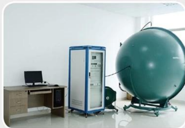
ullbrich sphere for testing luminous flux
