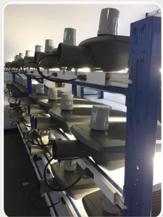
led street lighting aging
