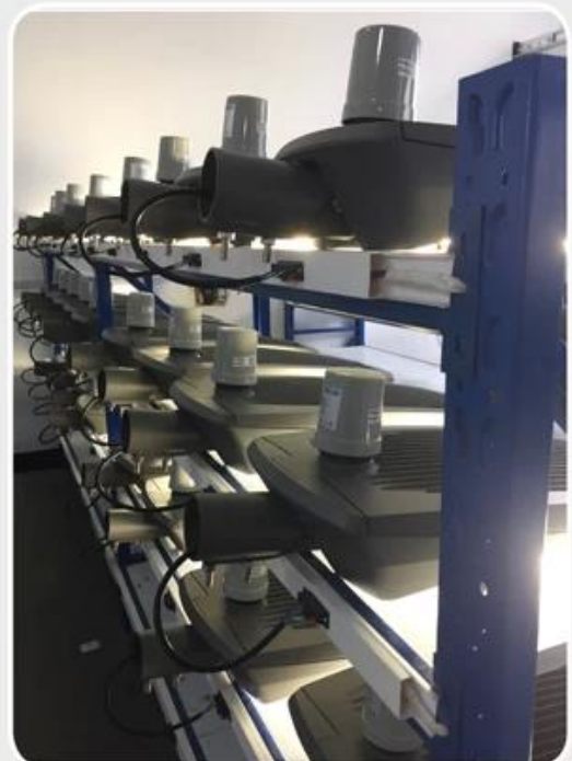
led street lighting aging testing line.
