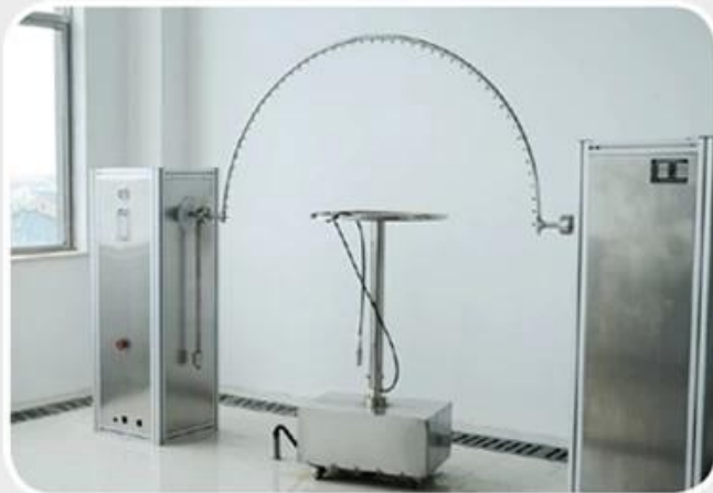
ingress protection (ip) testing equipment.
