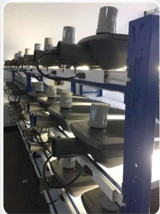
led street lighting aging testing line.
