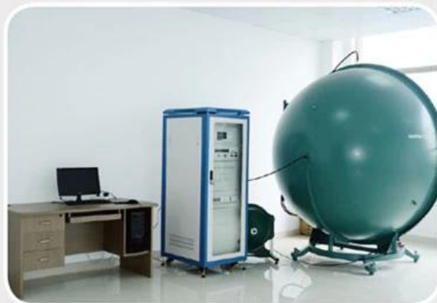
ullbrich sphere for testing luminous flux
