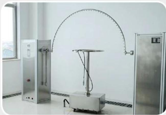
ingress protection (Ip) testing equipment.
