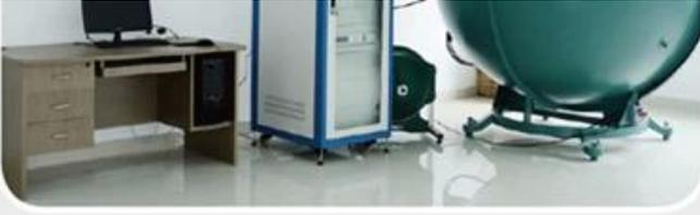
ullbrich sphere for testing luminous flux
