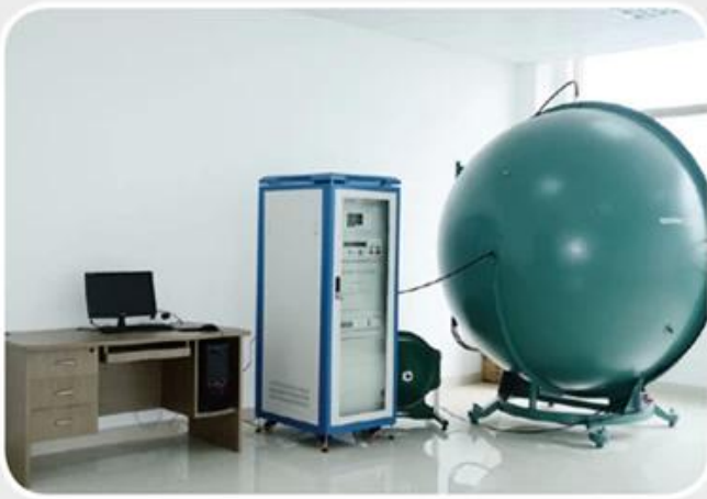
ullbrich sphere for testing luminous flux
