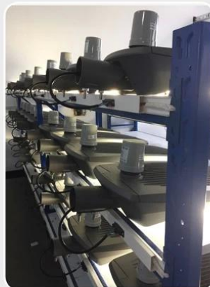
led street lighting aging testing line.
