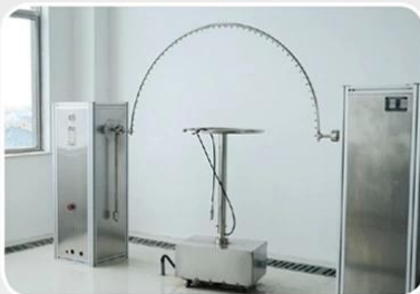
ingress protection (Ip) testing equipment.
