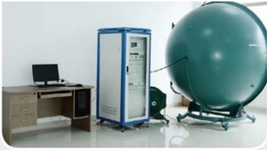
ullbrich sphere for testing luminous flux
