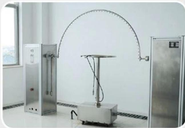
ingress protection (Ip) testing equipment.
