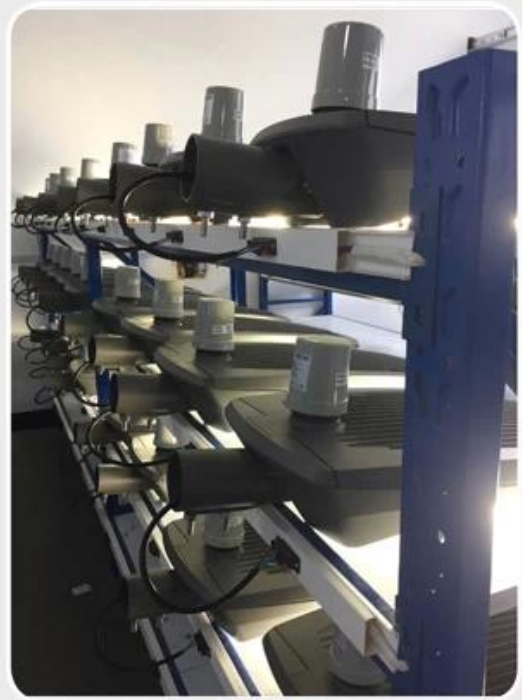
led street lighting aging testing line.
