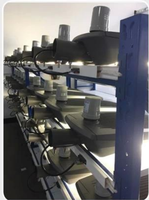
led street lighting aging testing line.
