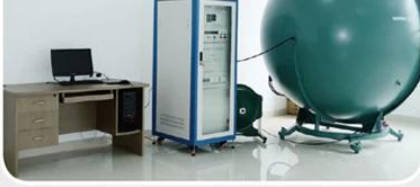
ullbrich sphere for testing luminous flux
