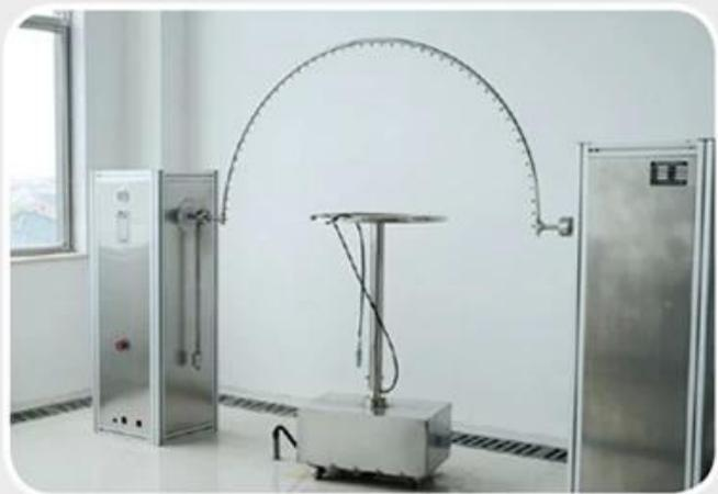
ingress protection (Ip) testing equipment.
