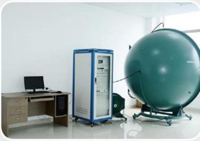
ullbrich sphere for testing luminous flux
