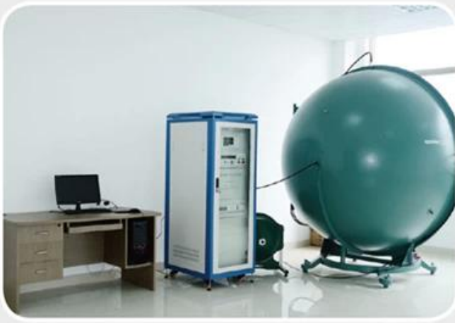
ullbrich sphere for testing luminous flux
