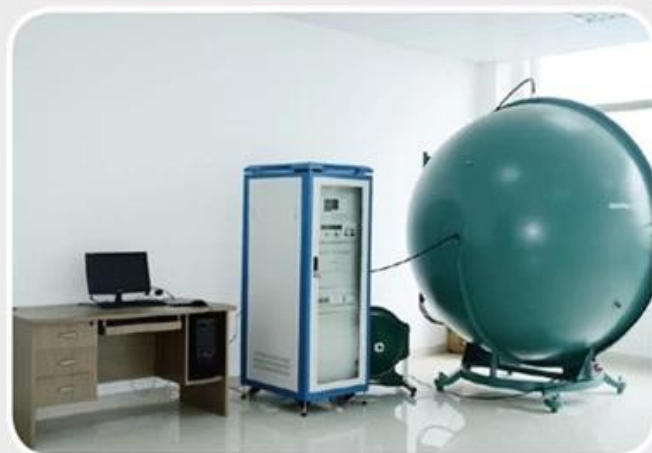
ullbrich sphere for testing luminous flux
