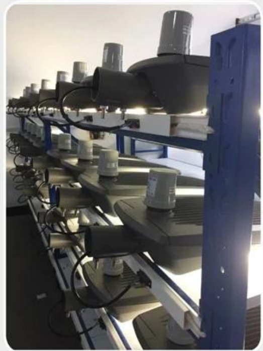
led street lighting aging testing line.
