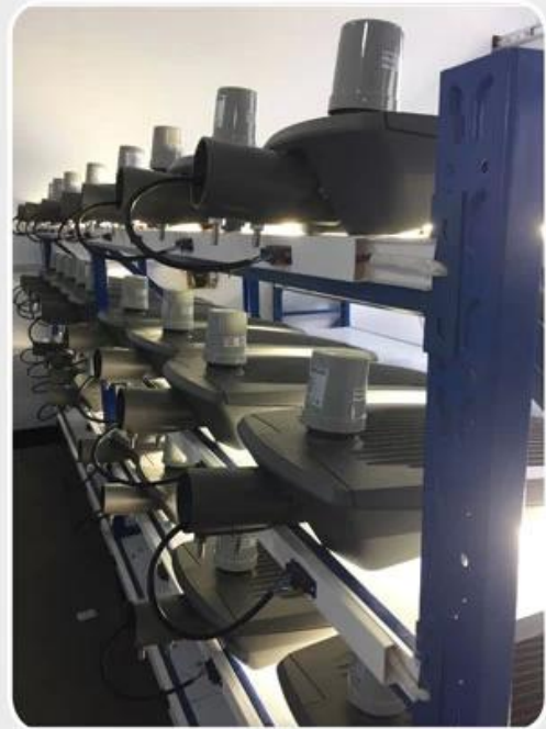
led street lighting aging testing line.
