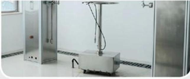
ingress protection (Ip) testing equipment.
