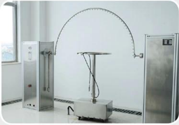
ingress protection (ip) testing equipment.
