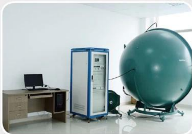
ullbrich sphere for testing luminous flux
