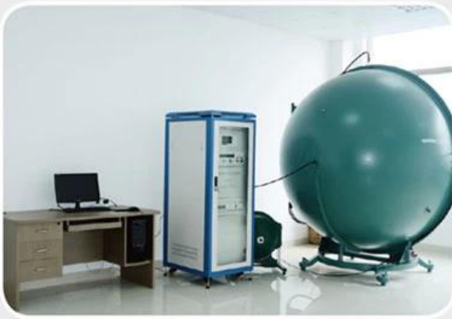
ullbrich sphere for testing luminous flux
