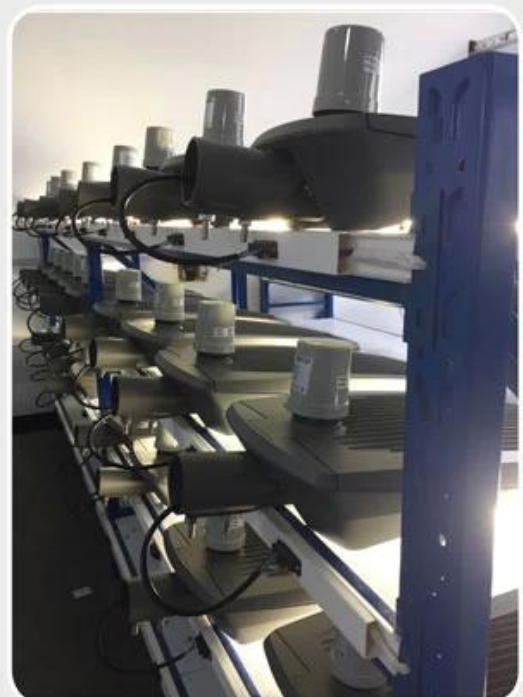
led street lighting aging testing line.
