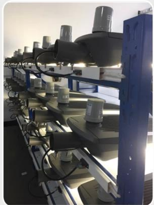
led street lighting aging testing line.
