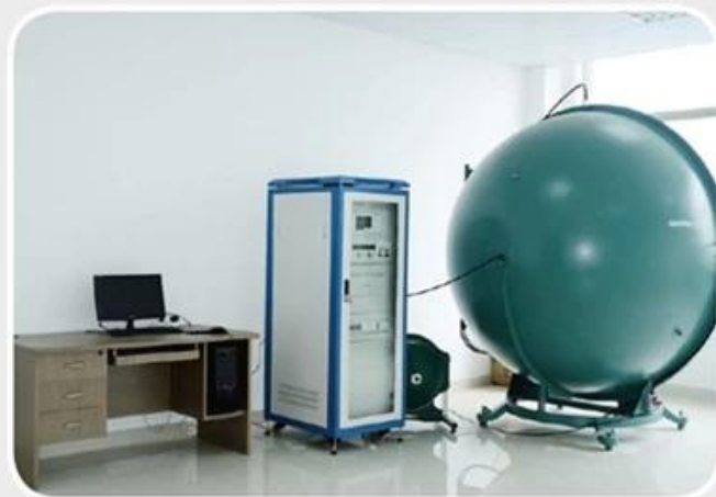
ullbrich sphere for testing luminous flux
