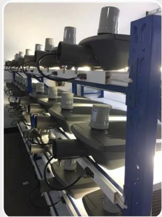
led street lighting aging testing line.
