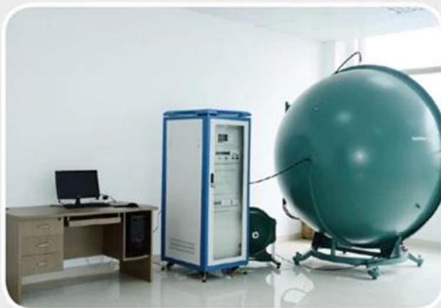
ullbrich sphere for testing luminous flux
