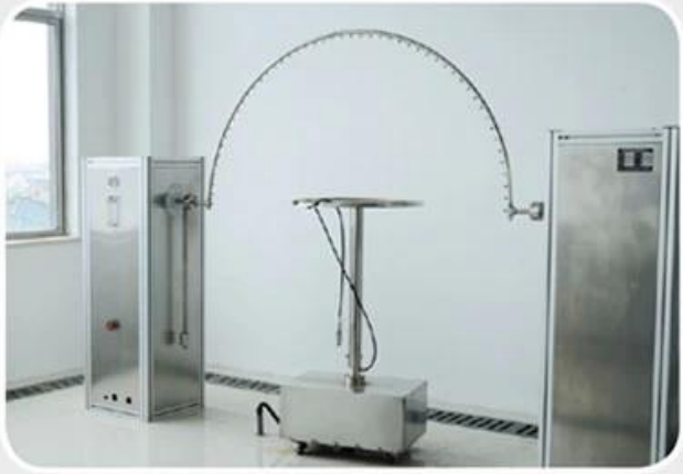
ingress protection (ip) testing equipment.
