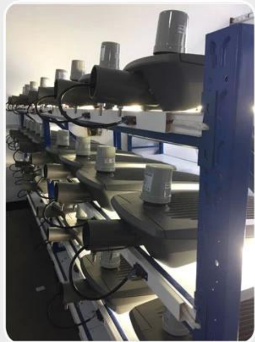
led street lighting aging testing line.
