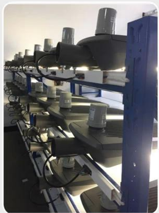
led street lighting aging
